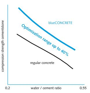
Water Cement Ratios between 0.2 and 0.55 can be driven with the blue CONCRETE-Technology > The compressive strength can be significantly increased while workability and material quality are improved with a cement reduction of 20%.
